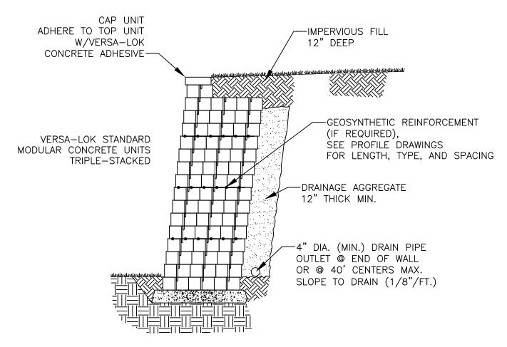
TYPICAL SECTION - TRIPLE-STACKED STANDARD UNIT RETAINING WALL
