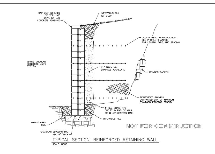
THESE PRELIMINARY DETAILS ARE INTENDED AS AN AID IN DESIGNING ATTRACTIVE, DURABLE RETAINING WALLS WITH VERSA-LOK STANDARD UNITS. FINAL DETERMINATION OF THE SUITABILITY OF ANY INFORMATION OR MATERIAL FOR THE USE CONTEMPLATED, AND ITS MANNER OF USE, IS THE SOLE RESPONSIBILITY OF THE USER. A FINAL PROJECT SPECIFIC DESIGN SHOULD BE PREPARED BY A QUALIFIED, LICENSED, PROFESSIONAL ENGINEER.
