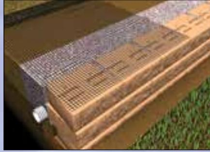
When the weight of the units alone is insufficient to resist soil loads, horizontal layers of VERSA-GRID or other types of geogrid are used to reinforce soil behind walls. VERSA-LOK retaining walls can be built to heights of 50 feet or more with proper soil reinforcement and design assistance from a licensed professional engineer.
