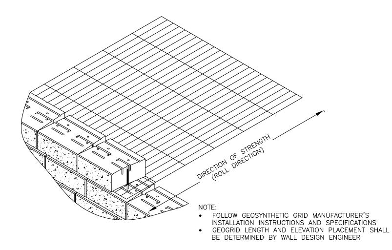
GEOSYNTHETIC INSTALLATION DETAIL
